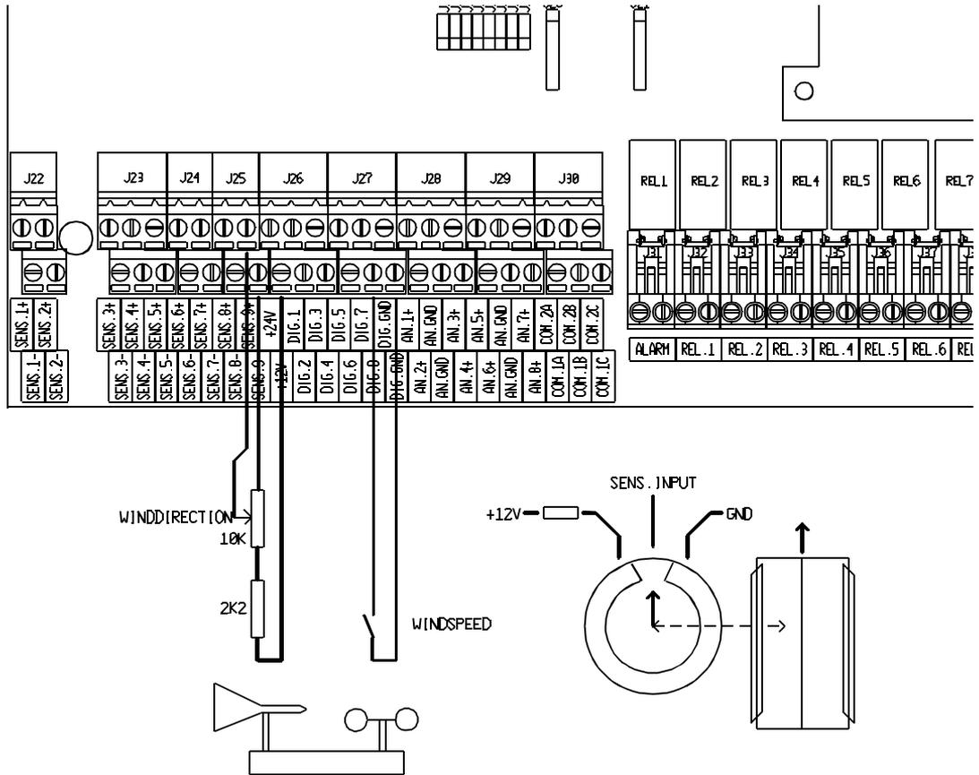
**Important!** To connect the weather station always use shielded cable with a minimum diameter of 0.8 mm<sup>2</sup> and mount the shielding only in the Navigator to terminal SENSOR min.
