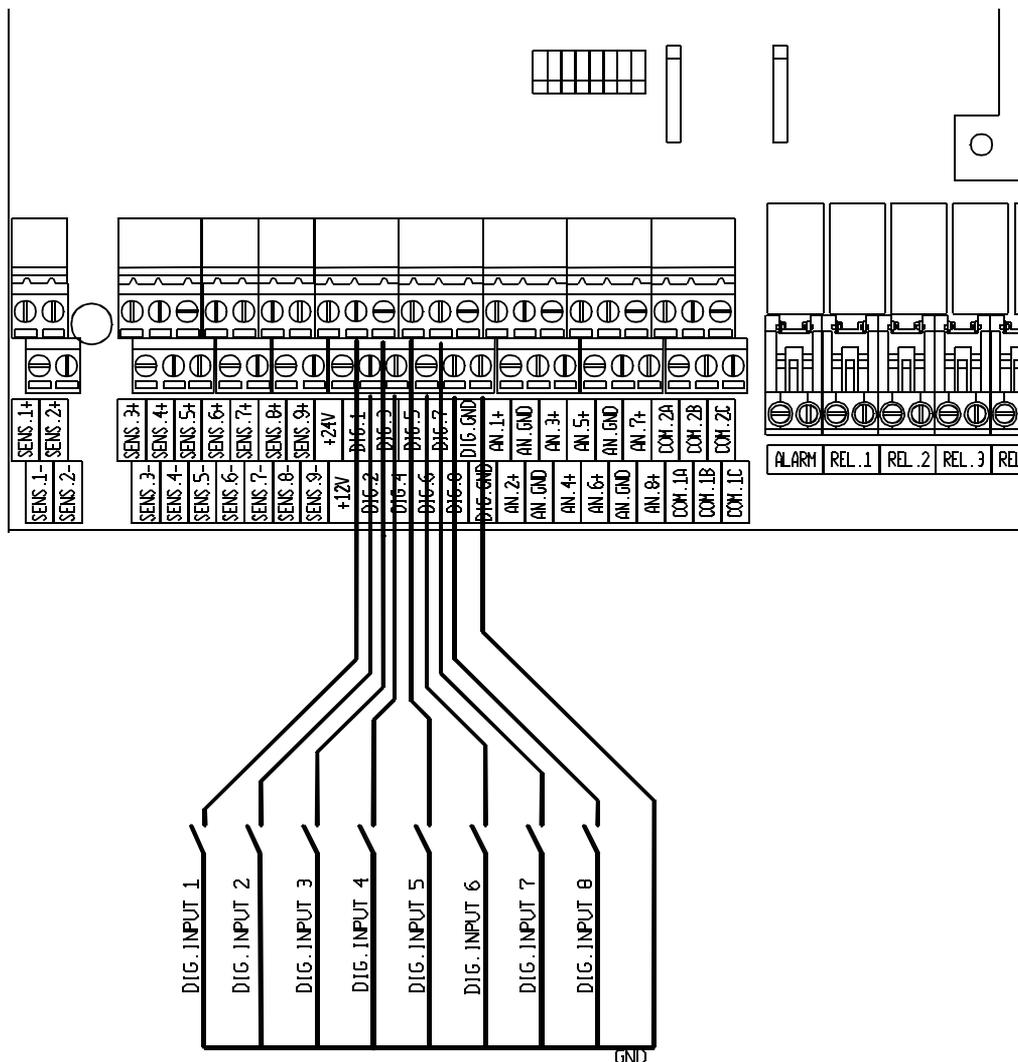
**Important!** To connect the feed and/or water counters always use shielded cable with a minimum diameter of 0.8 mm<sup>2</sup>. Connect the shielding in the Navigator to the DIG.GND terminal. Do not connect the shielding at the counter.
