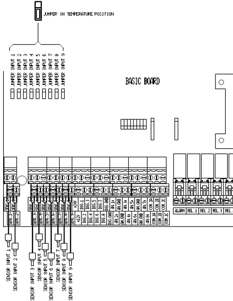
**Important!** To connect all sensor cabling always use shielded cable with a minimum diameter of 0.8 mm<sup>2</sup>. Connect the shielding in the computer always to the minus terminal of the corresponding sensor. Do not connect the shielding in the sensor.
