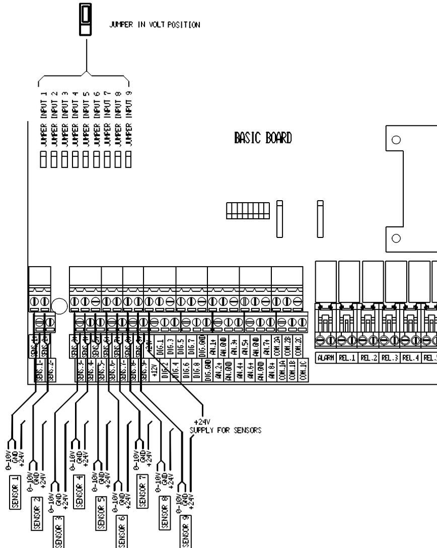
**Important!** To connect the humidity or CO2 sensors always use shielded cable with a minimum diameter of 0.8 mm<sup>2</sup>. Connect the shielding in the Navigator to the corresponding minus terminal. Do not connect the shielding in the sensor.
